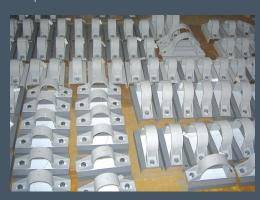
Fabricated pipe clamps for petrochemical pipe application.
