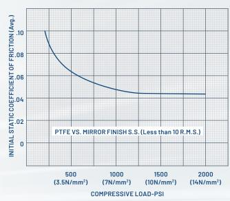
Note: Friction reduces as the compressive stress is increased.
