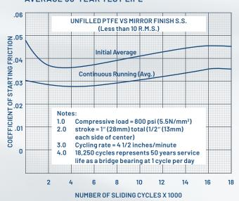
Note: Initial starting friction reduces to a run-in value under continuous sliding conditions.
